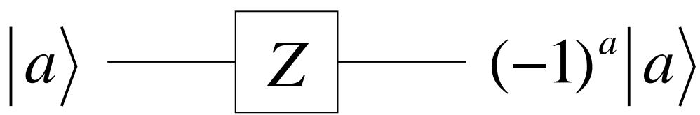
$$\begin{aligned} Z|0\rangle &= |0\rangle \\ Z|1\rangle &= -|1\rangle \end{aligned} \Leftrightarrow Z = \begin{bmatrix} 1 & 0 \\ 0 & -1 \end{bmatrix}$$
