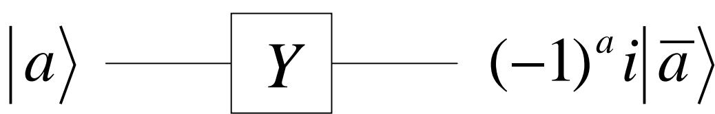
$$\begin{aligned} Y|0\rangle &= i|1\rangle \\ Y|1\rangle &= -i|0\rangle \end{aligned} \Leftrightarrow Y = \begin{bmatrix} 0 & -i \\ i & 0 \end{bmatrix}$$
