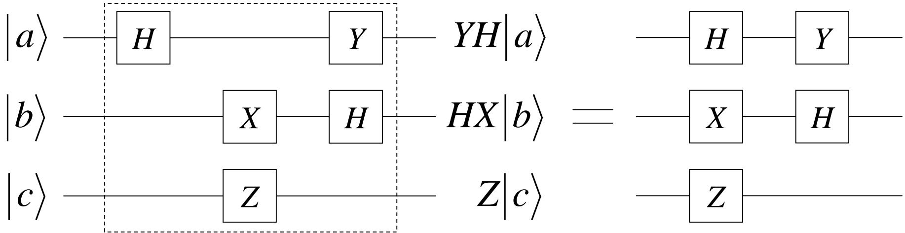
$$|a\rangle|b\rangle|c\rangle \xrightarrow{\underbrace{(YH \otimes HX \otimes Z)}_{U \text{ (8 by 8 unitary matrix)}}} (YH|a\rangle) \otimes (HX|b\rangle) \otimes Z|c\rangle$$
