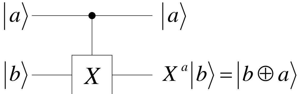
$$\begin{aligned} |b\rangle &= |b \oplus 0\rangle \text{ if } a = 0 \\ |\bar{b}\rangle &= |b \oplus 1\rangle \text{ if } a = 1 \end{aligned}$$
